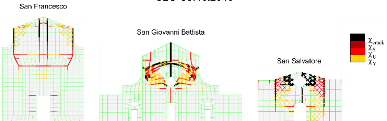
Figure 14. Damage patterns obtained for the three façades applying the three accelerograms with increasing values of the PGA: T0819-29.05.2012 (PGA=0.15g), MRN-20.05.2012 (PGA=0.26g), CLO-30.10.2016 (PGA=0.58g).
