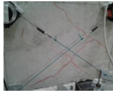
Figure 5. Diagonal cracks of the panel zone of the specimen J05 (Realfonzo et al. 2014).
