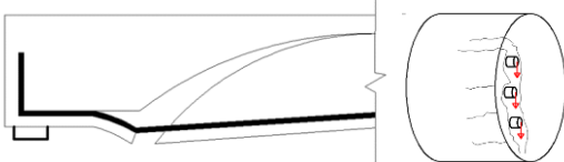
Figure 1. Overview of dowel action-effect contribute of sub-vertical longitudinal bars
