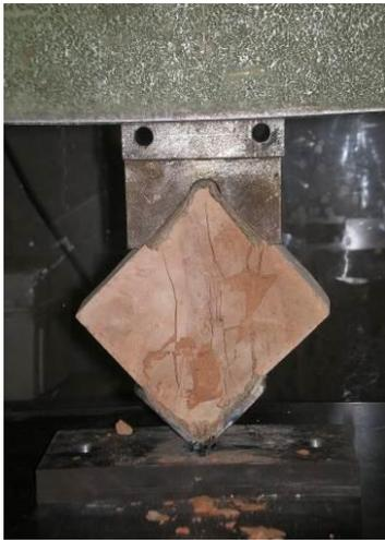
Figure 4. Square historic brick model under diagonal compression at failure.
