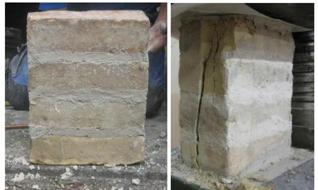
Figure 6. Brickwork wallette with historic brick.
