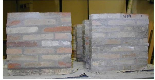
Figure 7. Wallettes with solid bricks in scale.
