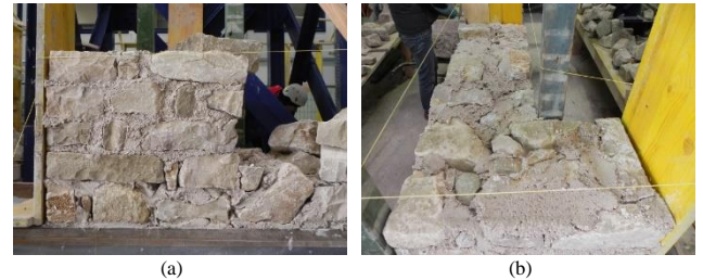
Figure 5. Masonry configuration: (a) front view, (b) horizontal section.
