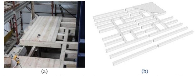
Figure 3. Second floor diaphragm: (a) orientation of beams and planks, (b) 3D rendering.
