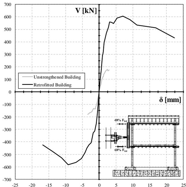
Figure 2: Lateral load-displacement envelopes.
