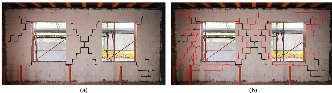
Figure 3: Final crack pattern of East façade at ground floor (inside view); reference (a) and retrofitted (b) building.
