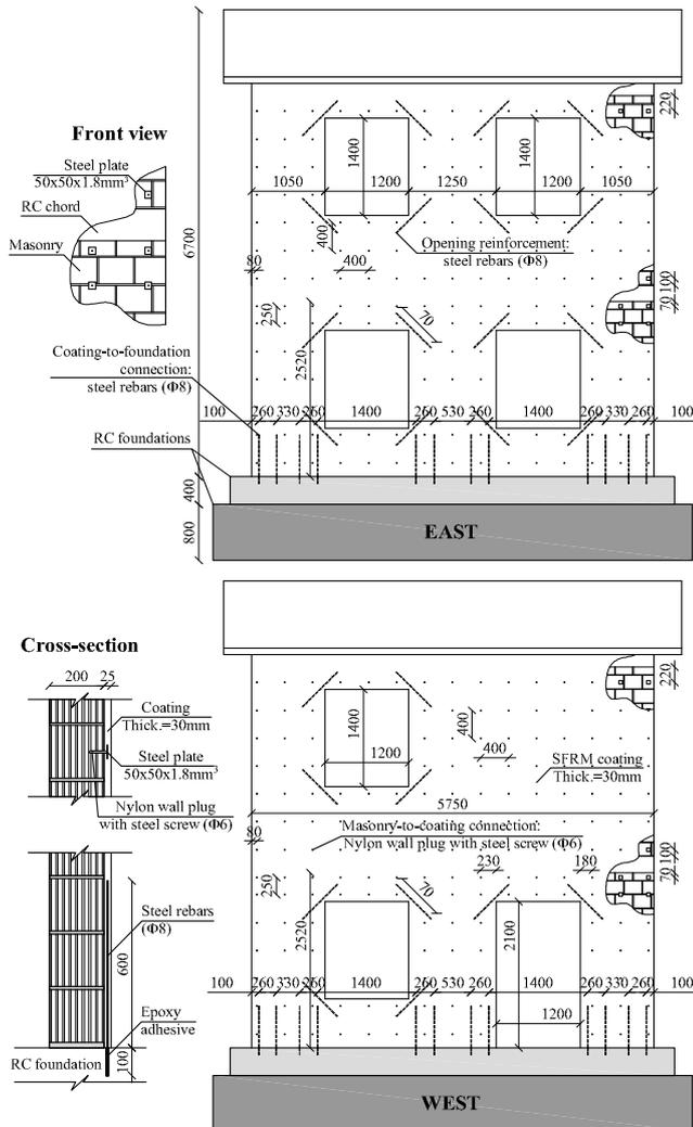
Figure 1: Main details of the retrofitting intervention.
