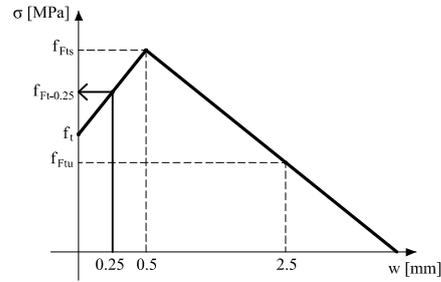
Figure 4: Bilinear uniaxial tensile stress-crack width law.
