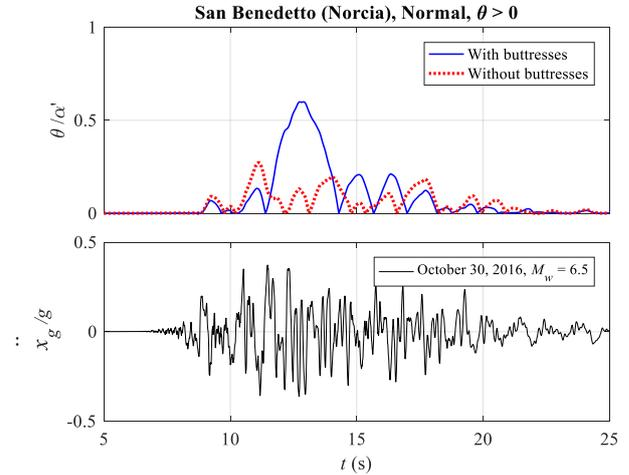
Figure 4. Time history of the one-sided rocking rotation response perpendicular to the San Benedetto façade for the October 30, 2016 accelerogram, considering both the presence/absence of buttresses.
