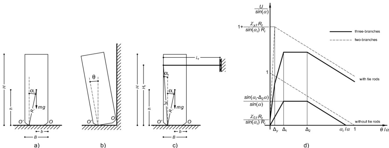
Figure 2. a) Geometrical parameters accounting for hinge indentation; b) One-sided displaced configuration ( $\theta > 0$ ); c) Geometrical parameters accounting for tie rods; d) Normalized moment–rotation relationship.
