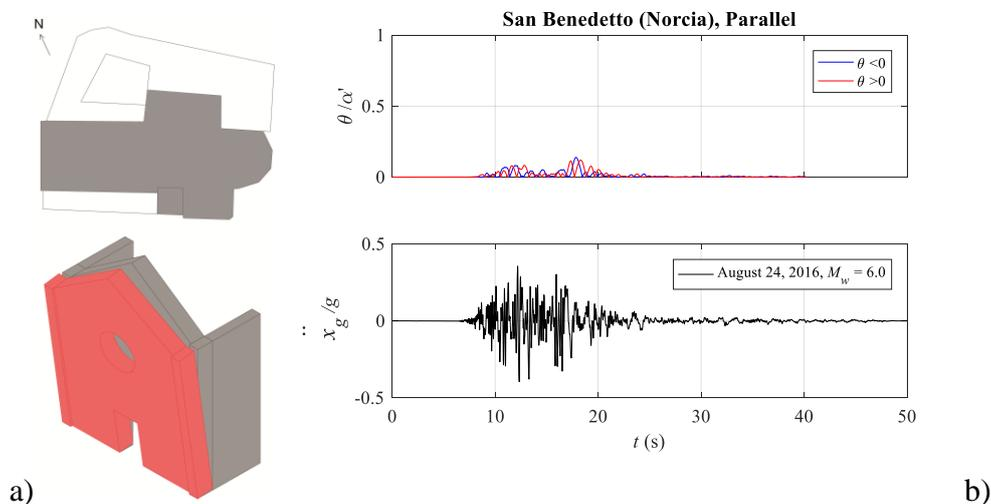
Figure 3. a) Model of the façade of San Benedetto (Norcia); b) Time history of the one-sided rocking rotation response parallel to the façade for the August 24, 2016 accelerograms.
