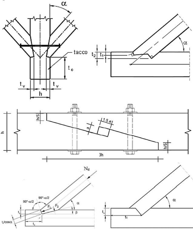
Figure 6. Carpentry joints.
