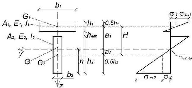
Figure 8. Reference cross-section for a composite beam with flexible connection and subjected to flexure, with corresponding distribution of normal stresses.
