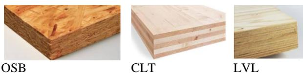
Figure 1. Example of timber based products.
