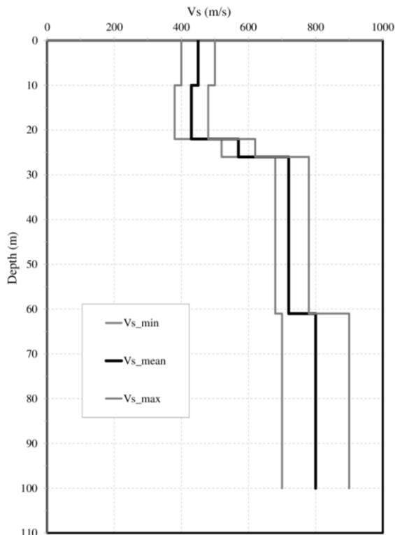
Figure 8: 1D profile of the mean shear wave velocity  $V_s$  from Down-Hole Test in Sesia river (black thick line) and ranges of variation assumed (grey thin lines).
