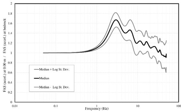
Figure 12: acceleration transfer function ratio: top to bedrock. Median value (black thick line); Median +/- Log Standard deviation (grey thin lines).
