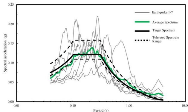
Figure 5: Acceleration response spectra of the seven selected real accelerograms for Sesia Area, scaled to a PGA 0.045g (949 years return period) and comparison with their mean response spectrum, structural damping 5%.
