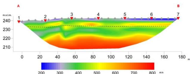
Figure 9: Seismic tomography performed in Sesia area, reporting the estimated depth of seismic bedrock. Note the dashed line representing the inversion in shear-wave velocity about at 10 m depth.
