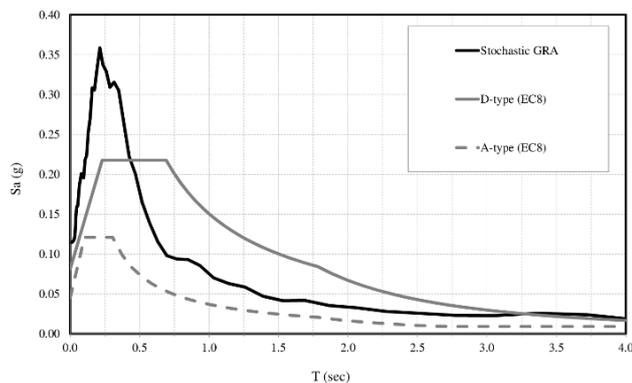
Figure 14: Response spectrum obtained from Stochastic GRA, in Sesia Area. Mean spectrum (black thick line) compared with the response spectra of EC8 for soil type: A and D, (dashed and continue grey line respectively).
