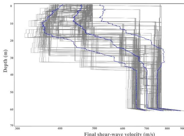
Figure 11: Variability of final shear wave velocity and layer thickness in the simulation carried out by STRATA. Median value (continue blue line); Median +/- Log Standard deviation (dashed blue lines); 1-350 realizations (grey lines).
