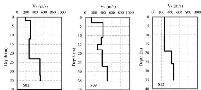
Figure 7: Shear wave velocity profiles from down-hole tests carried out along Pedemontana Piemontese alignment, according the following distribution: S02 – Rolino Area; S09 – Marchiazza Area; S12 – Torbola Area.
