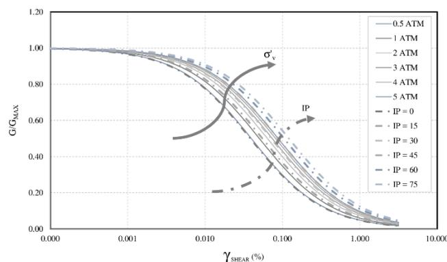
Figure 10: factors affecting degradation curves in Darendeli (2001) model, according to the value of Plasticity Index and Confining Pressure adopted in the present work.
