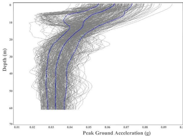
Figure 13: Peak Ground Acceleration profile, resulted by Stochastic GRA. Median value (continue blue line); Median +/- Log Standard deviation (dashed blue lines); 1-350 realizations (grey lines).
