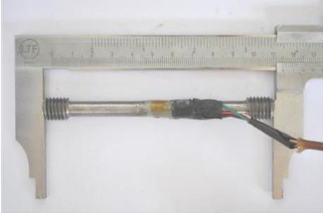
Figure 4. The instrumented steel specimen.
