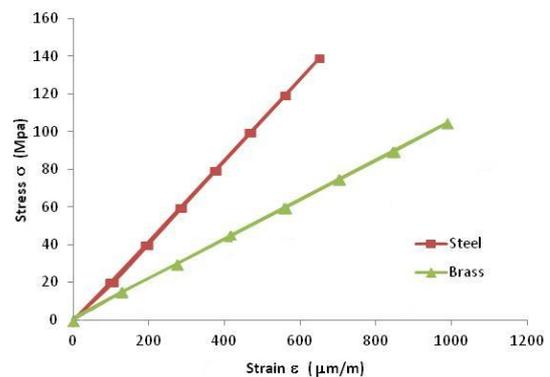
Figure 5. Experimental stress-strain curves obtained from tensile tests on the steel and brass specimens using the wired method.
