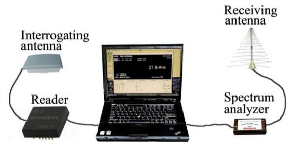
Figure 3. Scheme of the interrogation unit: a RFID reader and a spectrum analyzer connected to an antenna and to a personal computer.
