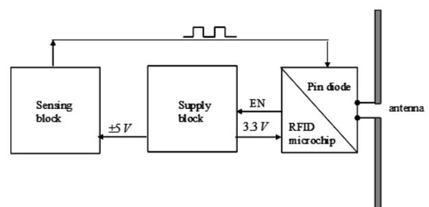
Figure 2. Scheme of the sensor tag, three main circuit blocks. The sensor tag is quiescent and can be activated on demand.
