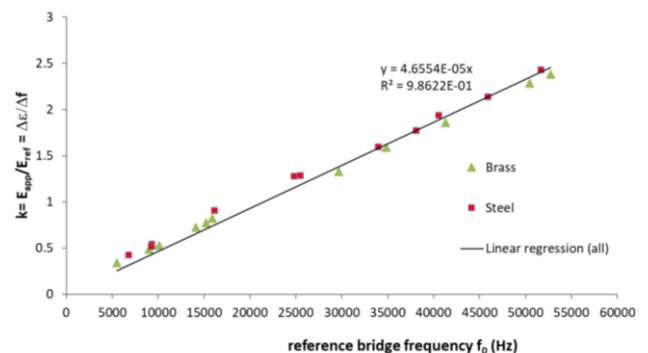
Figure 7. Experimental values for  $k = E_{app}/E_{ref}$  as function of the initial frequency  $f_0$ . Values of  $k$  also express the ratio among the real strain increment in the gauge ( $\Delta\varepsilon$ ) and the measured frequency variation  $\Delta f$ .
