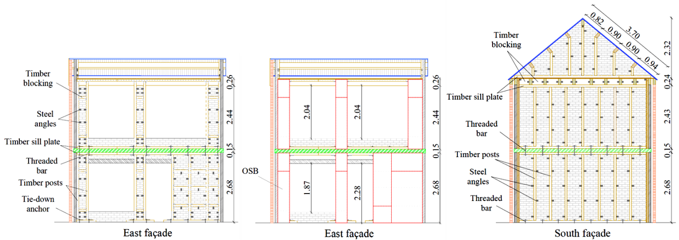
Figure 7. Retrofitting building elevations. Units of m.
