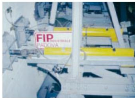
Figure 2- Shaking table test of SMADs (FIP Industriale)
