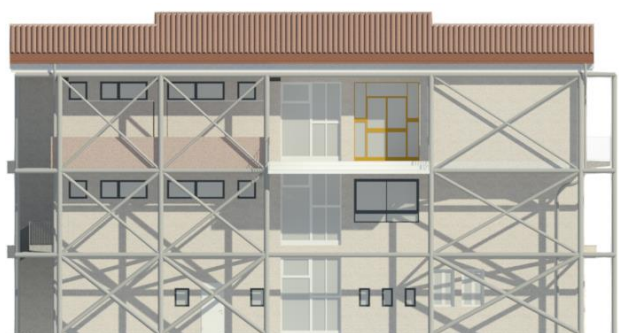
Figure 19 - Façade with exoskeletons in direction x . North Side: 2D//_CBF_X_Fz1_Fx1-1_N3.
