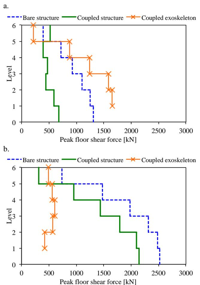
Figure 5. Profiles of peak floor shear forces on the bare existing structure and on the coupled system in: a.  $x$ -direction; b.  $y$ -direction. Life Safety limit state.
