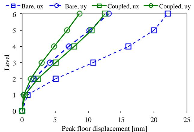
Figure 4. Profiles of peak floor displacements in  $x$ - and  $y$ -direction, comparisons between bare existing structure and coupled system. Life Safety limit state.
