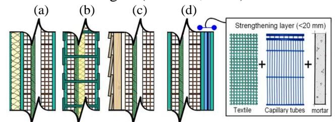
Figure 6. Construction details to combine energy efficiency and minimize damage to infill walls
