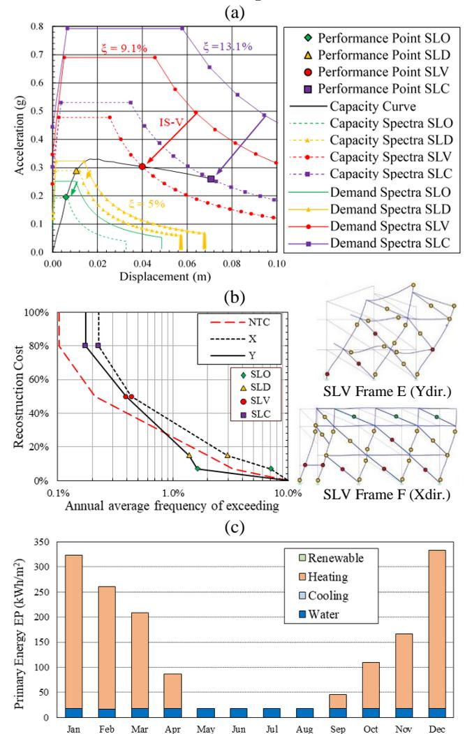
Figure 2. Seismic-Energetic Assessment of the Case study building: (a) Capacity vs. Demand within an Acceleration-Displacement-Response-Spectrum (ADRS); (b) (Seismic) Expected Annual Losses - EALs; (c) Global Energy consumption, EP<sub>gl</sub>, and its contributions.
