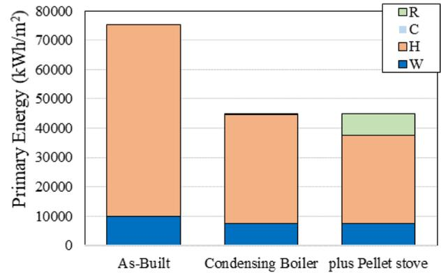
Figure 4. HVAC system Energetic Retrofit, Yearly Global Energy consumption, EP<sub>gl</sub>
