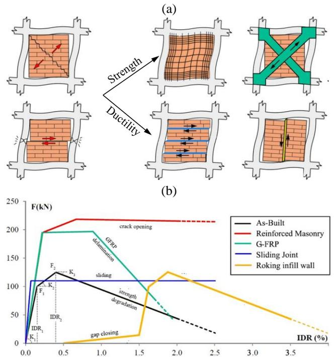
Figure 5. (a) Strength and Ductility seismic retrofit strategies on infill-wall; (b) equivalent strut capacity of infill walls in the as-built or retrofitted configuration
