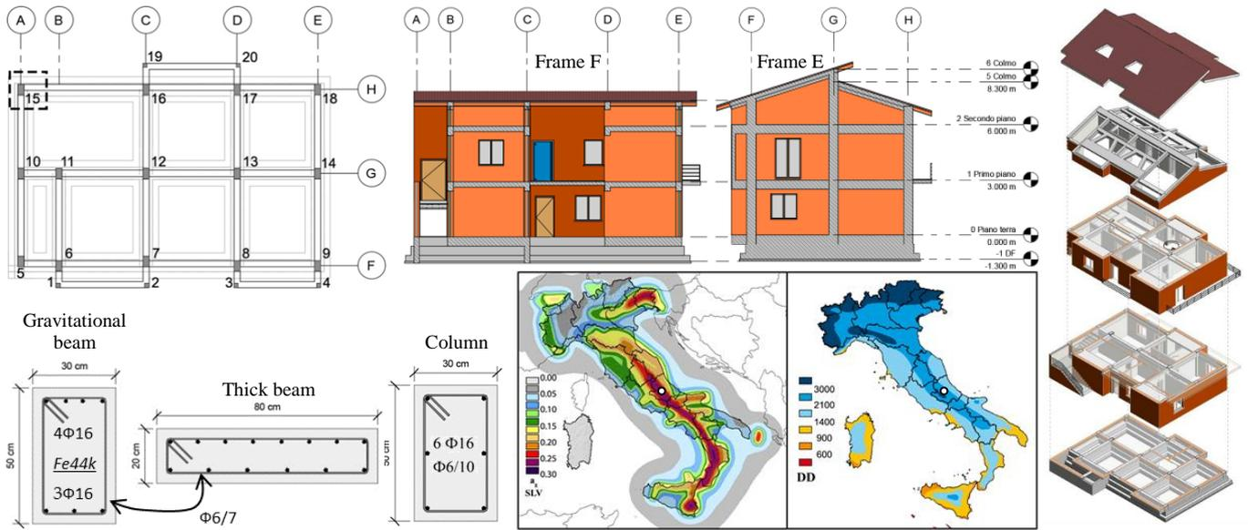
Figure 1. Characterization of the case study: foundation plan; frame section; exploded axonometry; main structural beam and column sections at the interface with the joint panel zone; geographical location (seismic hazard and climate demand).
