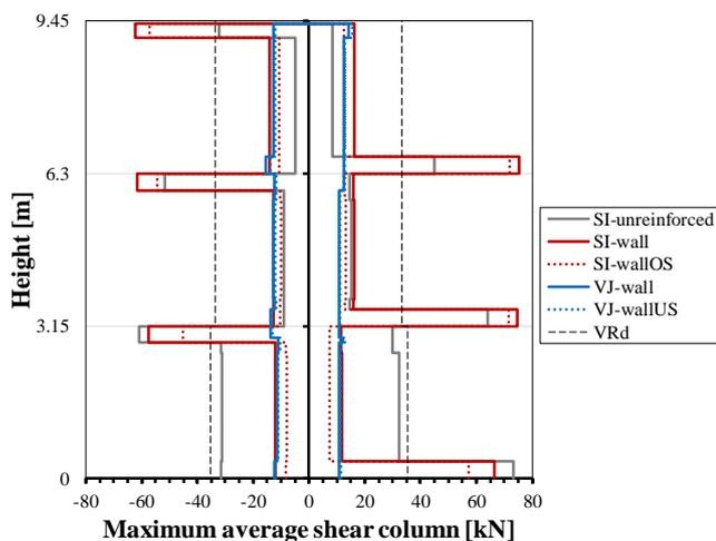
Figure 10. Results of the time-history analyses: maximum average shear demand in the column A.
