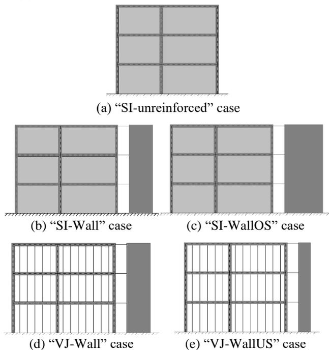
Figure 3. Schematic of the different configurations considered in the study.
