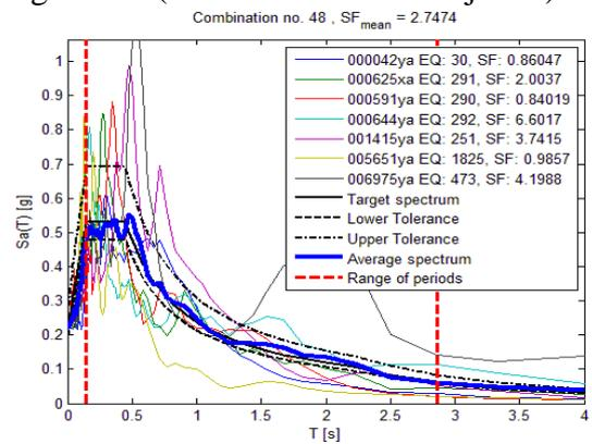
Figure 7. Selection of 7 spectrum-compatible ground motions for the time history analysis.
