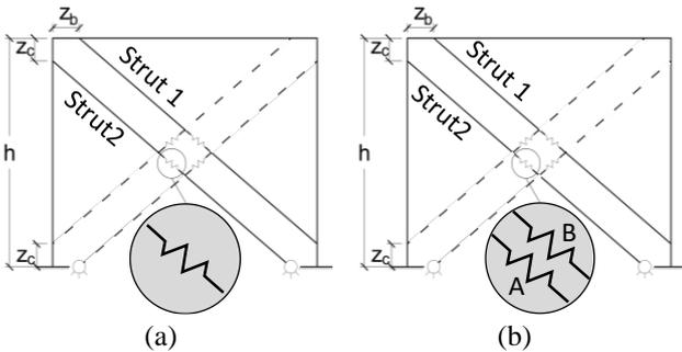
Figure 5. Schematic of the simplified models for the solid infill ("SI") (a) and the "downgraded" infill ("VJ") (b).
