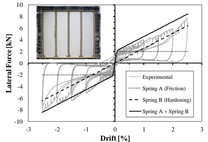
Figure 4. Infill “downgrade: experimental results obtained in (Preti and Bolis, 2017a) -vs.- equivalent double-strut model calibration.
