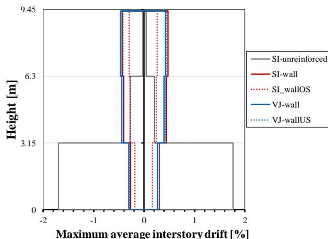
Figure 9. Results of the time-history analyses: maximum average inter-story drift along the frame height.
