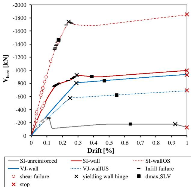
Figure 6. Results of the non-linear static analyses.
