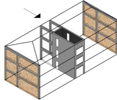
(a) layout of the seismic-resisting system in the transversal direction
