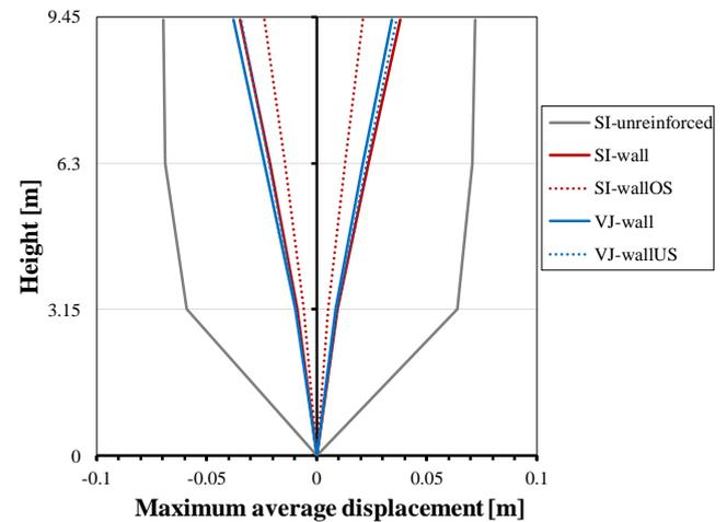
Figure 8. Results of the time-history analyses: maximum average displacement along the frame height.
