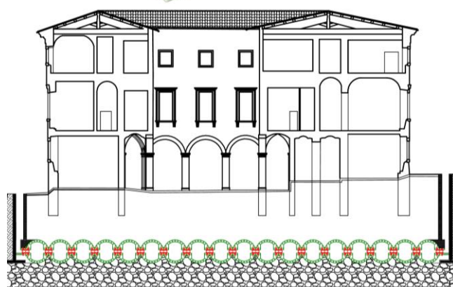
Figure 6. Axonometric and transversal cross-sections of the isolation system proposed for Palazzo Margherita, L'Aquila (Structural design L. Marchetti and C. Lufrano, Consultant for base isolation: P. Clemente and A. De Stefano, Company: IRPCO SpA Roma).
