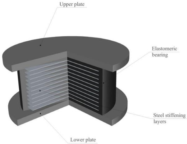
Figure 3. Components of a rubber bearing isolator
