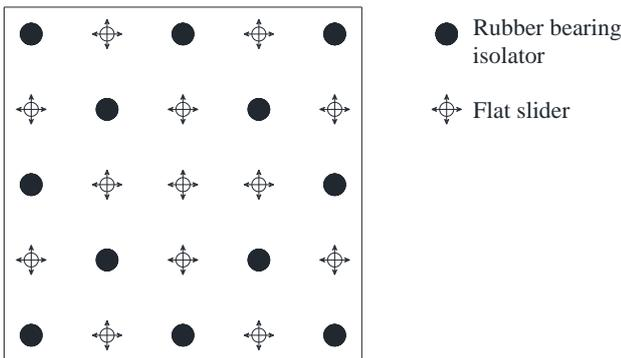
Figure 4. Isolation devices layout
