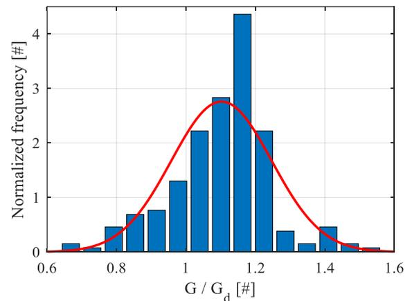
Figure 5. Experimental variability of shear modulus for rubber bearings
