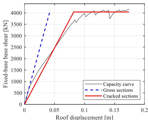
Figure 2. Capacity curves of the fixed-base building
