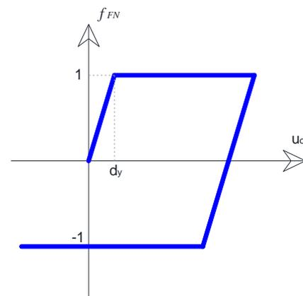
Figure 6. Normalized friction force
