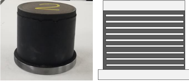
Figure 1. Small scale HDRB test piece: picture of a specimen (left), and cross-section (right)
