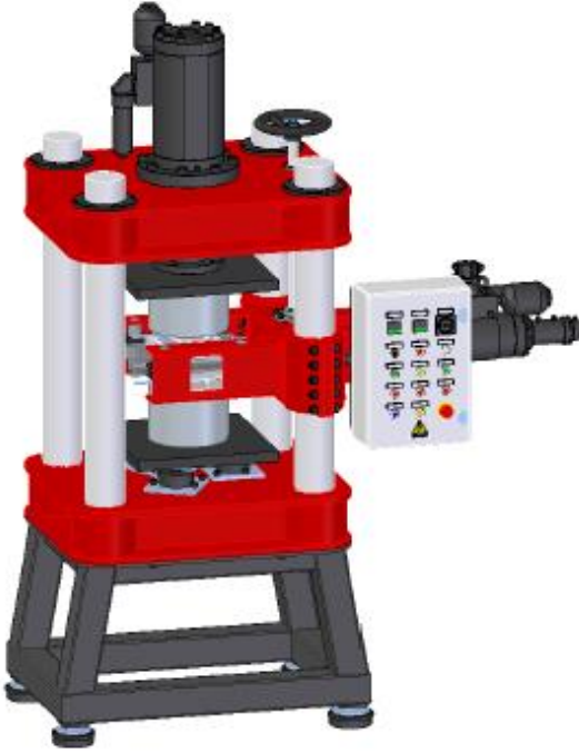
Figure 2. Schematic view of the biaxial test set-up
