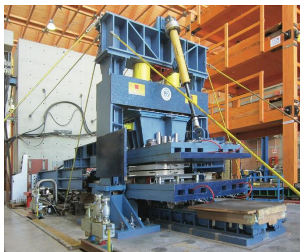
Figure 7. The bearing tester system at University of Basilicata
