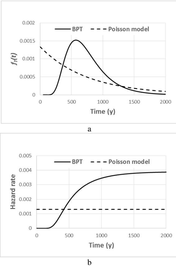
Figure 1 (a) Probability density functions of interarrival time and (b) hazard rates for the Poisson model and the Brownian Passage Time model.
