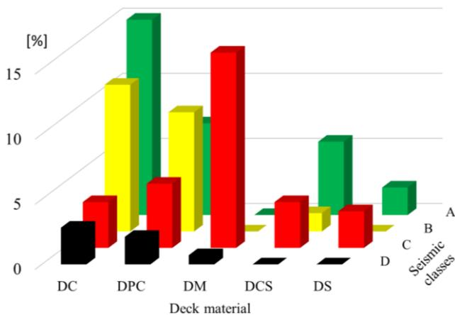
Figure 12. Seismic classification by deck material.
