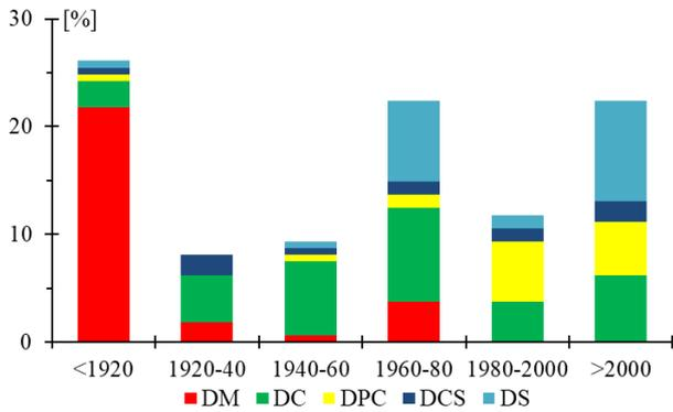
Figure 9. Distribution of structural materials over the years [Masonry (DM); Reinforced Concrete (DC); Prestressed Reinforced Concrete (DPC); Composite steel (DCS) and Steel (DS)].
