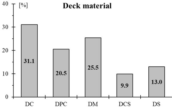
Figure 3. Statistical distribution of the deck materials. [Reinforced Concrete (DC), Prestressed Reinforced Concrete (DPC), Masonry (DM), Composite steel (DCS) and Steel (DS)]
