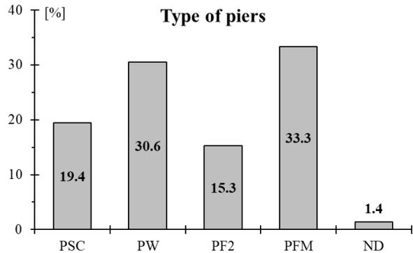
Figure 8. Statistical distribution of the type of piers. [Single Column (PSC), Wall (PW), Frame - Double (PF2), Frame - Multi (PFM) and Not available (ND)]
