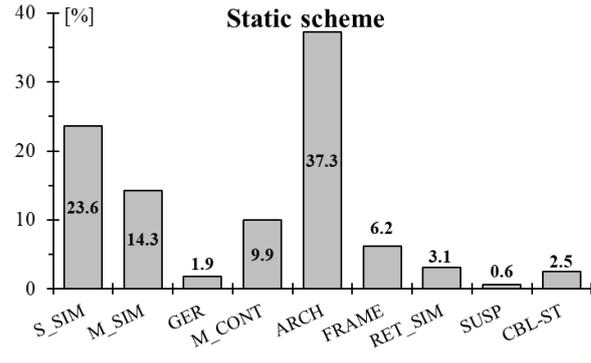
Figure 4. Statistical distribution of the static schemes. [single span simply (S\_SIM), multi-span simply (M\_SIM), multi-span Gerber scheme (M\_GER), multi-span continuous (M\_CONT), arch (ARCH), frame (FRAME) reticular simply supported (RET\_SIM), suspended (SUSP) and cable-stayed (CBL-ST)]
