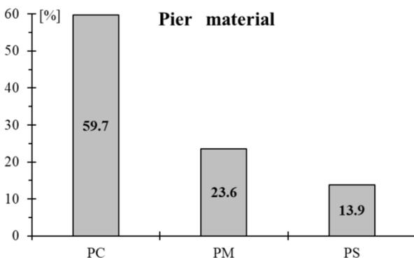
Figure 7. Statistical distribution of the pier material. [Reinforced Concrete Piers (PC), Masonry Piers (PM) and Steel Piers (PS)]
