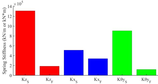
Figure 3. Representative values of footing and longitudinal strip beam stiffnesses (S: Strip beam, F: foundation)
