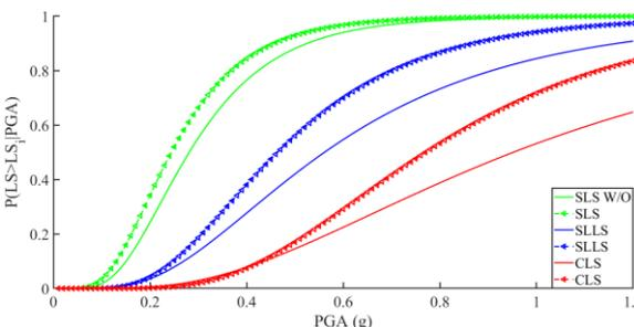
Figure 7. FFs for beams W/O & W/ SSI (linear) in decoupled case.
