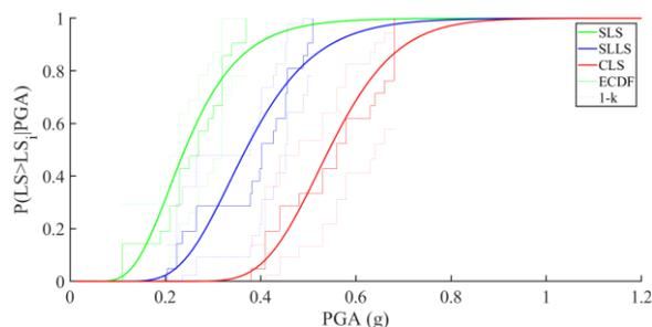
Figure 10. Pipes W/O SSI, decoupled, Greenwood's 95% confidence level ( $k=0.05$ ).
