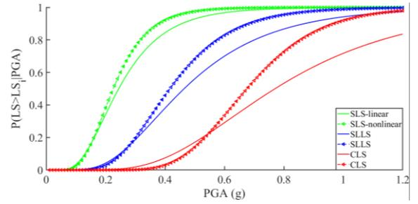
Figure 8. FFs for beams W/ linear and nonlinear SSI in decoupled case.
