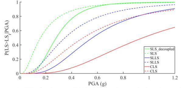
Figure 9. FFs for beams W/O SSI in decoupled and coupled case.
