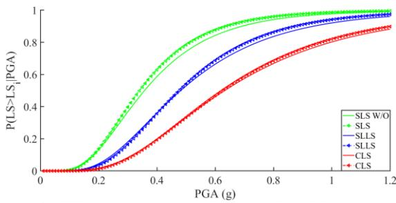
Figure 6. FFs for columns W/O & W/ SSI (linear) in decoupled case.
