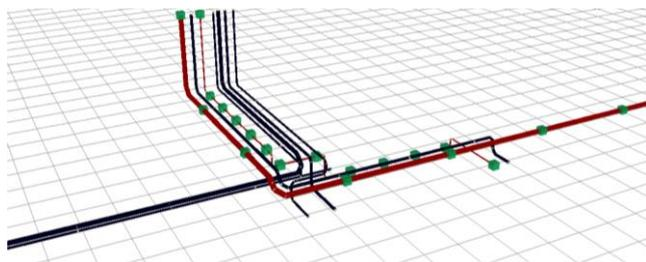
Figure 2. The piping system model in (SeismoSoft 2018). The BCs are also highlighted with green.
