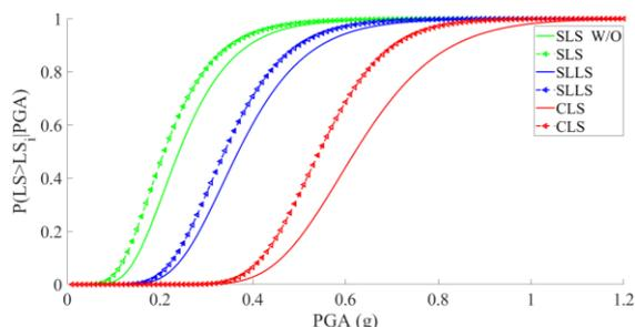
Figure 11. Pipes W/O & W/ linear SSI in decoupled case.
