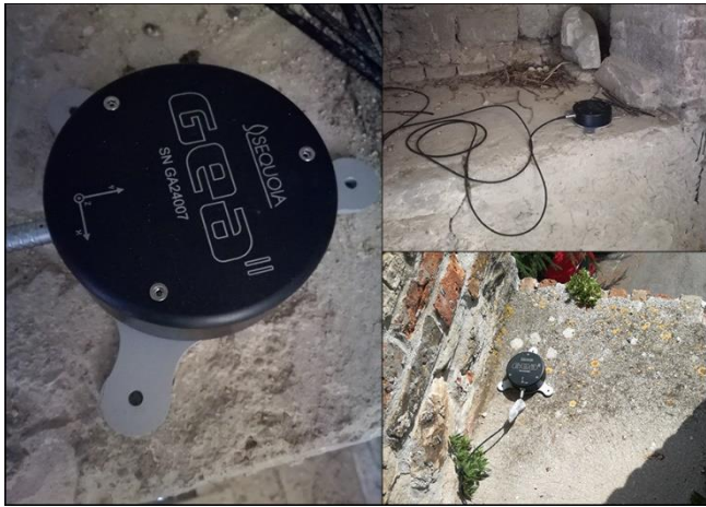
Figure 5. Views of the used equipment for the AVS of the civic clock tower of Rotella (AP).
