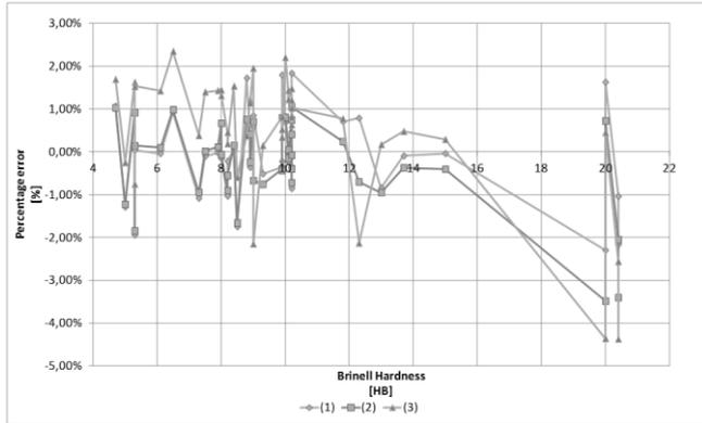
Figure 8. Percentage errors with respect to the envelope curve of the ASTM whole table (Legend - 1: envelope from tables; 2: partial envelope; 3: total envelope)
