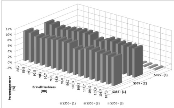
Figure 16. Percentage errors in predicting the Brinell Hardness for S355 steels (UNI ISO standard) (Legend - 1: envelope from tables; 2: partial envelope; 3: total envelope)
