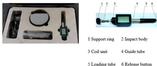
Figure 6. The MH100 Leeb hardness tester.
