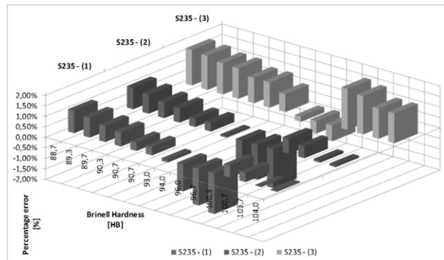
Figure 9. Percentage errors in predicting the Brinell Hardness for S235 steels (ASTM standard) (Legend - 1: envelope from tables; 2: partial envelope; 3: total envelope)
