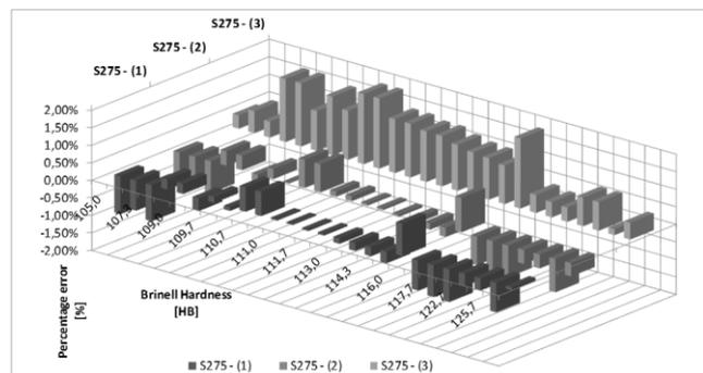
Figure 10. Percentage errors in predicting the Brinell Hardness for S275 steels (ASTM standard) (Legend - 1: envelope from tables; 2: partial envelope; 3: total envelope)
