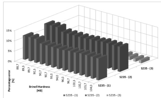
Figure 14. Percentage errors in predicting the Brinell Hardness for S235 steels (UNI ISO standard) (Legend - 1: envelope from tables; 2: partial envelope; 3: total envelope)
