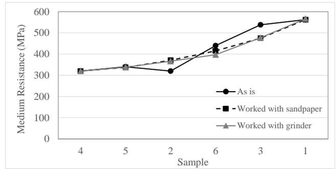
Figure 20. Medium tensile strengths of samples derived from the ASTM A370 standard according to the Rockwell scale.
