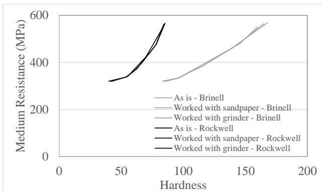
Figure 24. Average tensile strength vs. hardness curves of tested samples.
