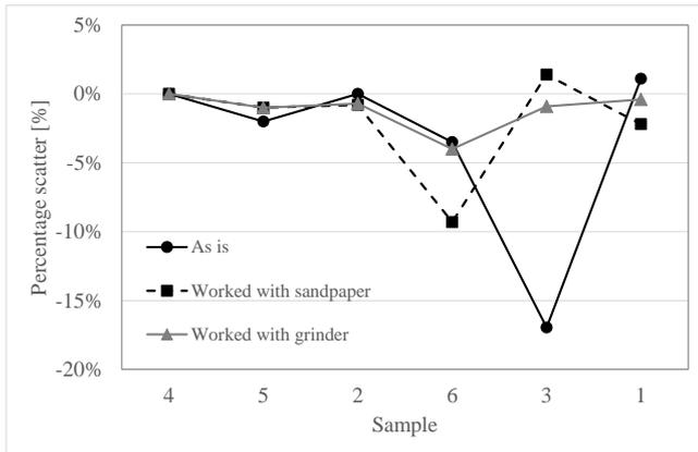
Figure 23. Percentage scatters between resistances derived from the Brinell scale hardnesses and the Rockwell scale ones.
