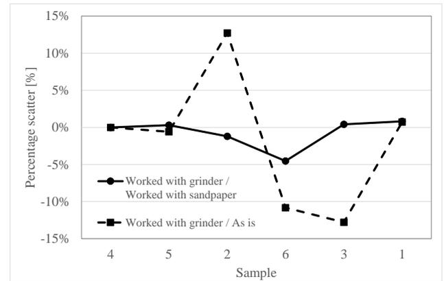
Figure 22. Percentage scatters among medium tensile strengths of samples derived from the Rockwell scale.
