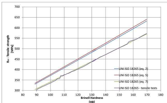
Figure 12. Comparison among hardness-strength curves (Brinell method – UNI ISO 18265 standard; tensile tests curve from conversion tables)
