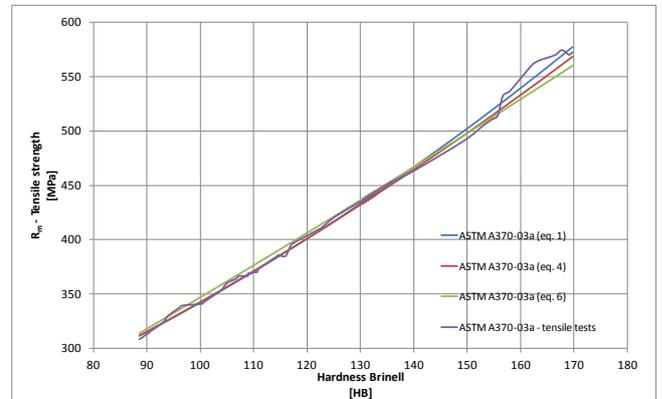
Figure 7. Comparison among hardness-strength curves (Brinell method – ASTM A370-03a standard; tensile tests curve from conversion tables).
