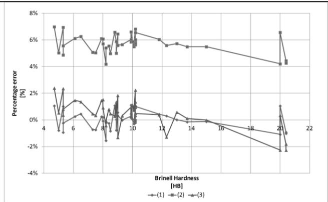
Figure 18. Percentage errors with respect to the envelope curves of the complete tables from ASTM and UNI ISO standards (Legend - 1: envelope from tables; 2: partial envelope; 3: total envelope)
