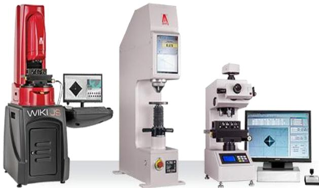
Figure 1. Instrumentations used for Rockwell (a), Brinell (b) and Vickers (c) hardness tests
