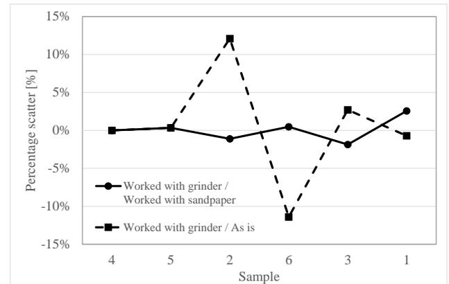
Figure 21. Percentage scatters among medium tensile strengths of samples derived from the Brinell scale.
