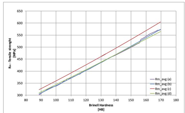
Figure 17. Comparison among hardness-strength curves deriving from average values between ASTM standard and UNI ISO one (Brinell method)
