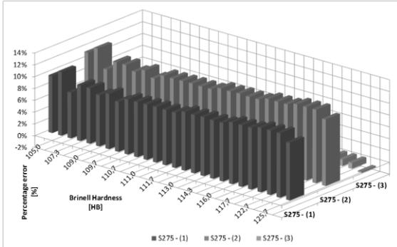
Figure 15. Percentage errors in predicting the Brinell Hardness for S275 steels (UNI ISO standard) (Legend - 1: envelope from tables; 2: partial envelope; 3: total envelope)
