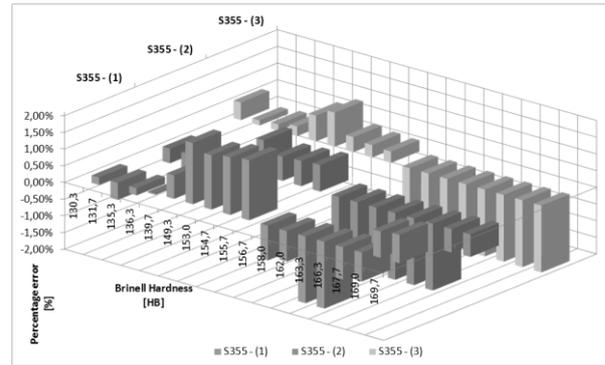
Figure 11. Percentage errors in predicting the Brinell Hardness for S355 steels (ASTM standard) (Legend - 1: envelope from tables; 2: partial envelope; 3: total envelope)
