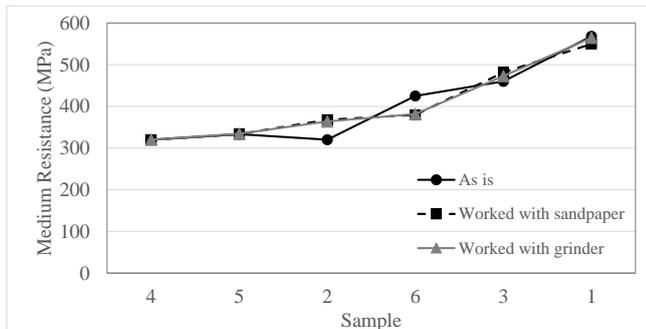
Figure 19. Medium tensile strengths of samples derived from the ASTM A370 standard according to the Brinell scale.
