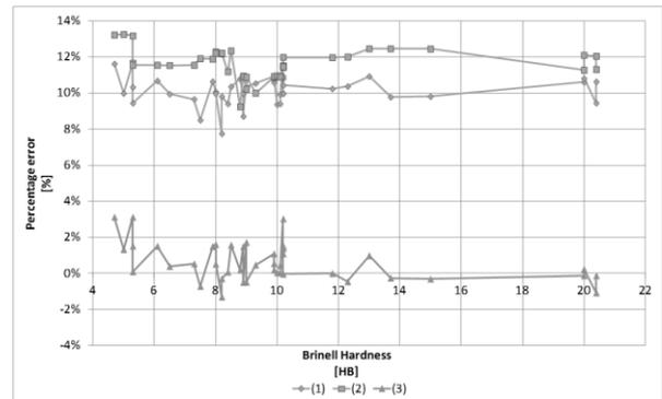
Figure 13. Percentage errors with respect to the envelope curve of the UNI ISO whole table (Legend - 1: envelope from tables; 2: partial envelope; 3: total envelope)
