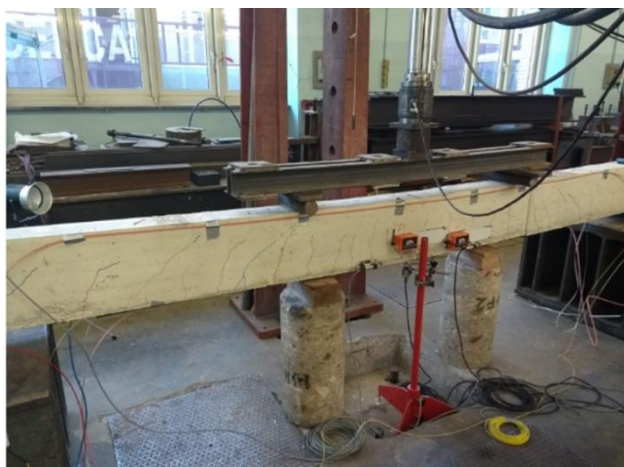
Figure 7. Cracks on tested beam.
