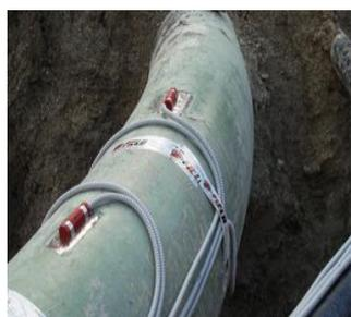
Figura 7. Strain Gauges
