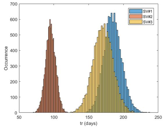
Figure 6. Distribution of maximum recovery time of seismic damage scenario SV1, SV2 and SV3.
