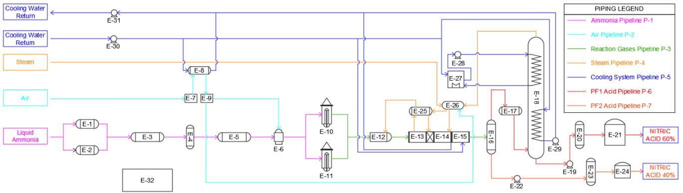
Figure 3. Process Flow Diagram of nitric acid plant.
