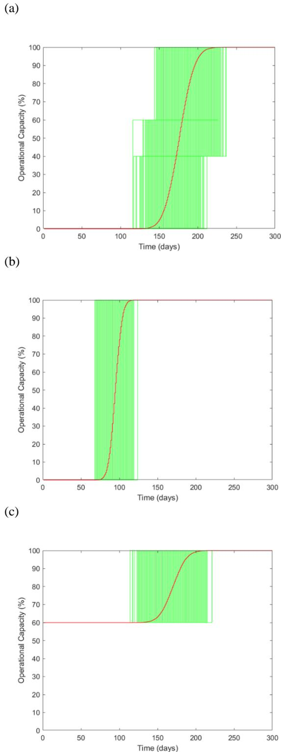
Figure 5. Probabilistic recovery curve of seismic damage scenario: (a) SV#1; (b) SV#2 and (c) SV#3.
