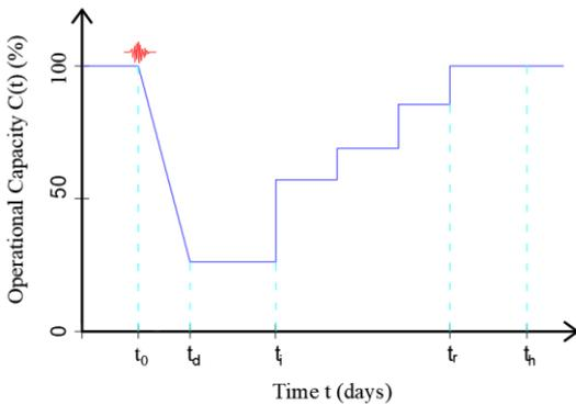
Figure 1. Plant operational capacity curve.
