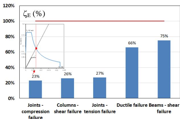
Figure 3. Seismic performance assessment of the case study building in terms of  $\zeta_E$  for each type of failure.
